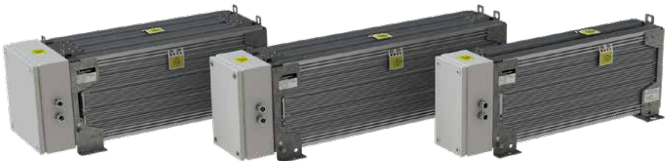
CMQ types with B-box IP54, quadruple, triple and double housings 2 cable glands M25 for resistor connection, 1 cable gland M12 for thermal switch
