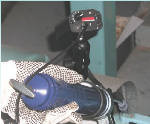
The Ultraprobe 201 Grease Caddy SWIVELS left/right and up/down for difficult angles
