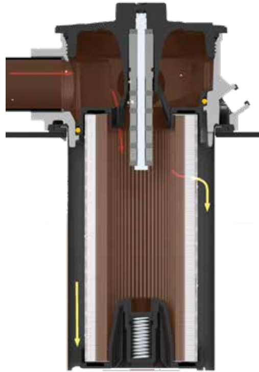
Magnetic pre-filtration and in-to-out filtration
