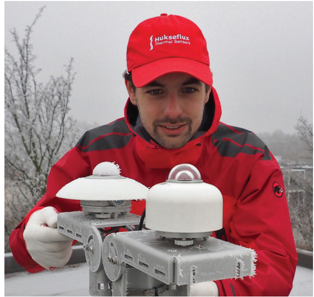
SR30 digital pyranometer with RVH™ technology (foreground), extreme winter weather conditions
