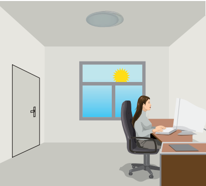
The light turns off completely when artificial light is not required, even with presence.
