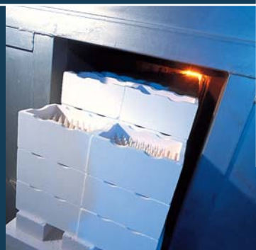
The baking of the ceramic components takes place 24 hours a day at a temperature of 1,650 °C.
