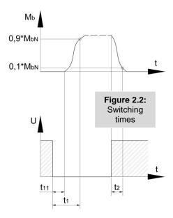
$\mathbf{t_2}$  = disconnection time = time between the switching on of the current and the ceasing of the braking torque ( $M_b \le 0.1*M_{bN}$ )
