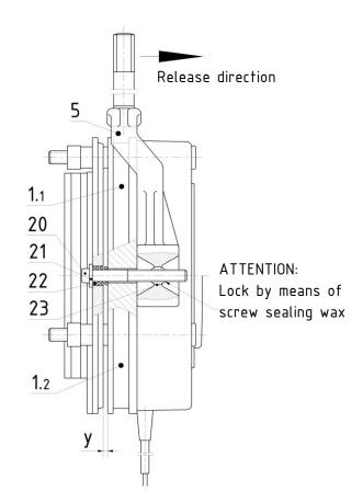
Figure 3.2: Assembly of the manual release (partial sectional view)
